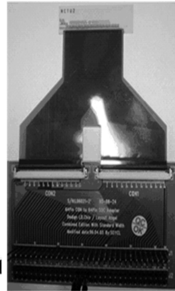
Fig. 2.7 The fabricated on-panel circuit for analog pixel memory and the corresponding measurement setup.
