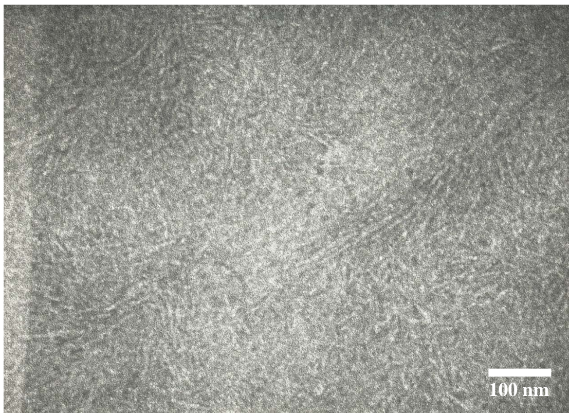
Figure 4-11. Transmission electron micrograph of the cryo-microtomed film of the pure PAU stained with \text{RuO}_4 . The dark region (matrix) corresponds to the phase of hard segments—PAU; the white region corresponds to the excluded PEG soft segment. The scale bar represents 100 nm.
