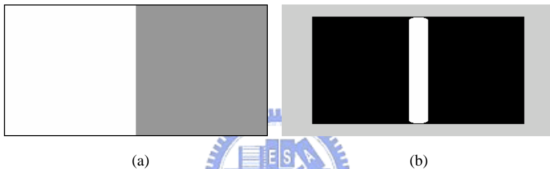
Fig.3-3 an example demonstrating coarse boundary detected by 1st-order feature (a) input image; (b) boundaries detected
