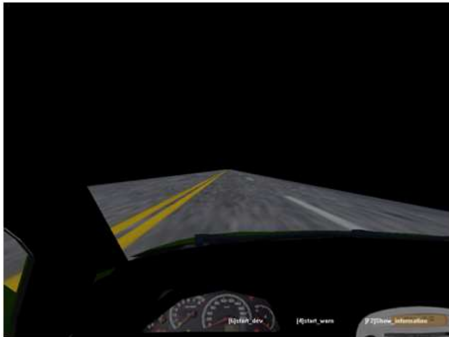
Fig. 2-4: The overview of surrounded VR scene. The VR-based highway scenes are projected into surround screen with seven projectors.
