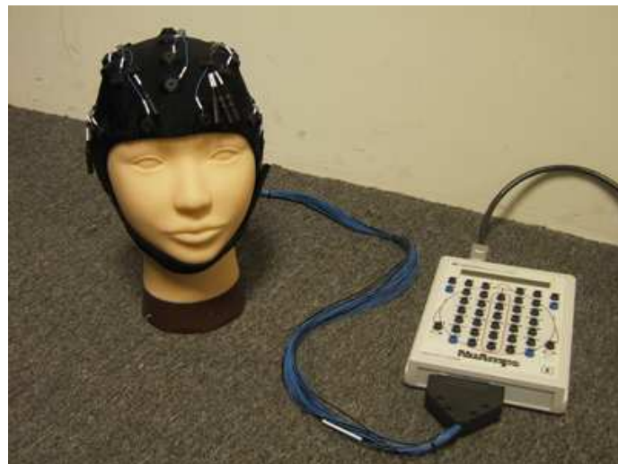
Fig. 1-3: Scan NuAmps Express system (Compumedics Ltd., VIC, Australia)
