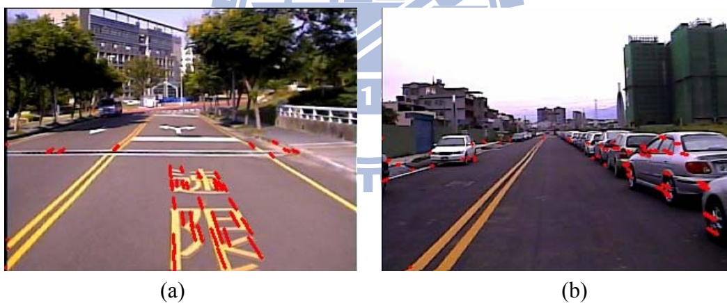
Fig. 4-2 Results of corner detection and its corresponding optical flow
