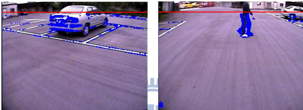
Fig. 4-18 results of image difference between current image and compensated image
