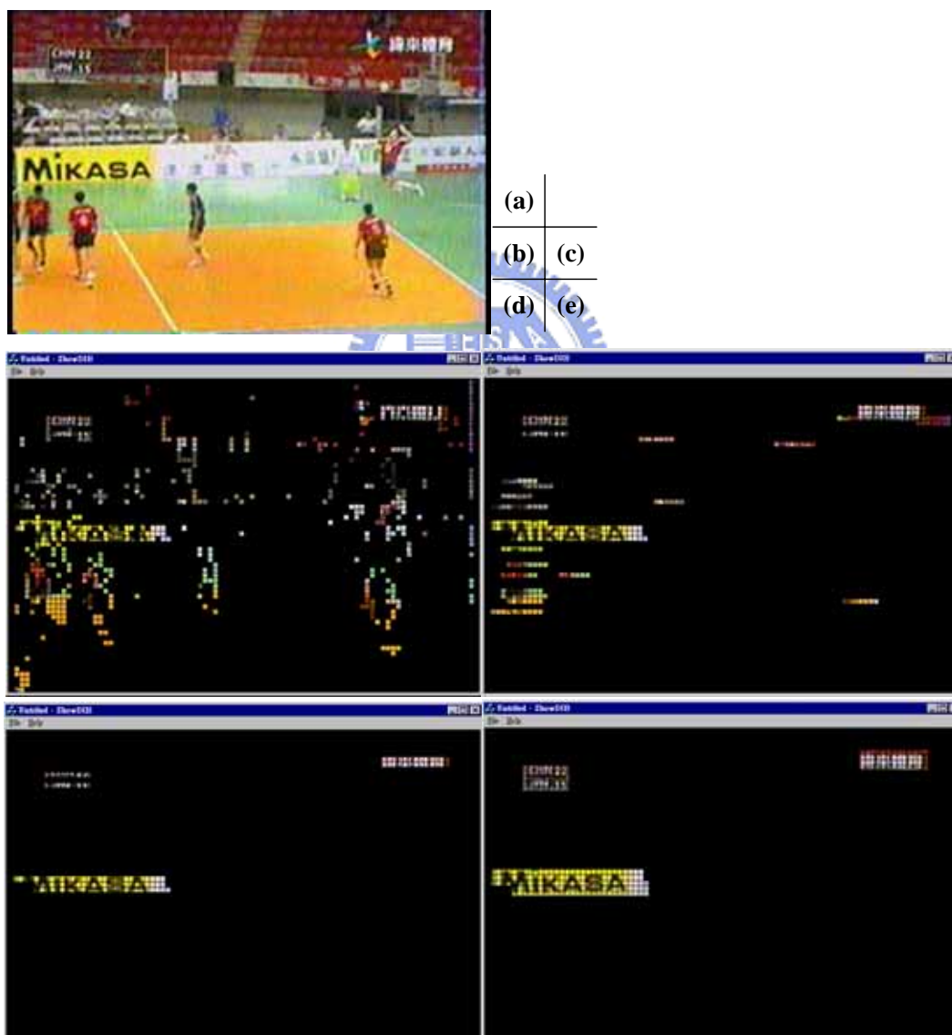
Fig. 4-10. Closed caption localization; (a) original I-frame; (b) result after filtering by horizontal gradient energy; (c) result after morphological operation; (d) result after filtering by SOM-based algorithm; (e) result after dilation
