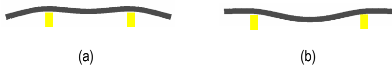
Figure 2-18 Schematic of (a) PDMS posts are placed too close to center.
