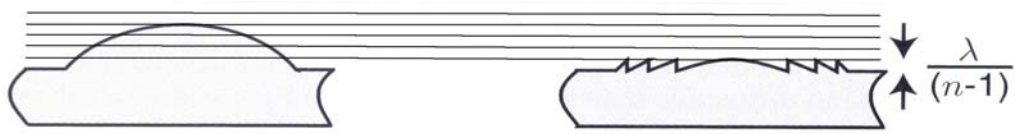
Figure 1-13: The blazing of a lens results in a reduced thickness.
