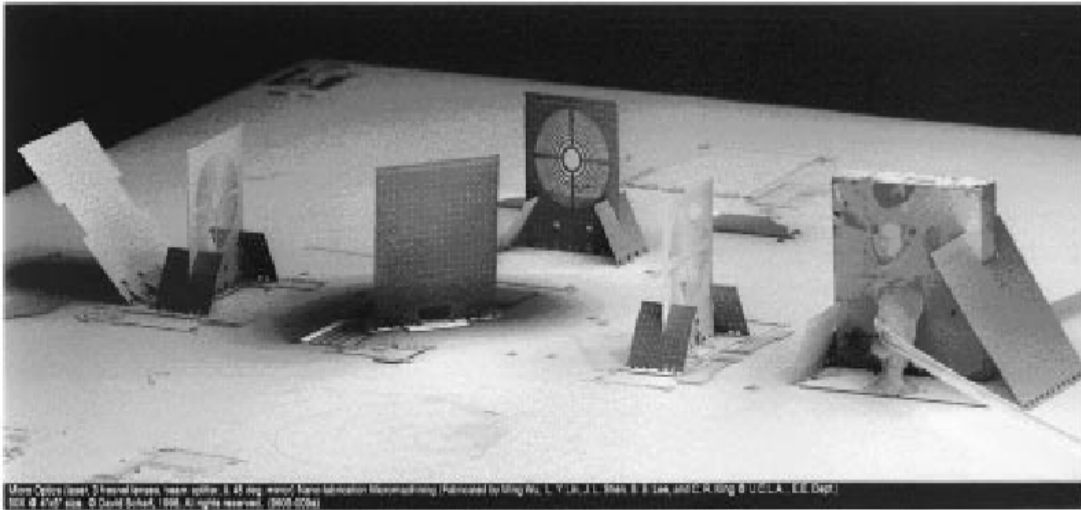
Figure 1-2: SEM micrograph of the monolithic optical-disk pickup head [3].
