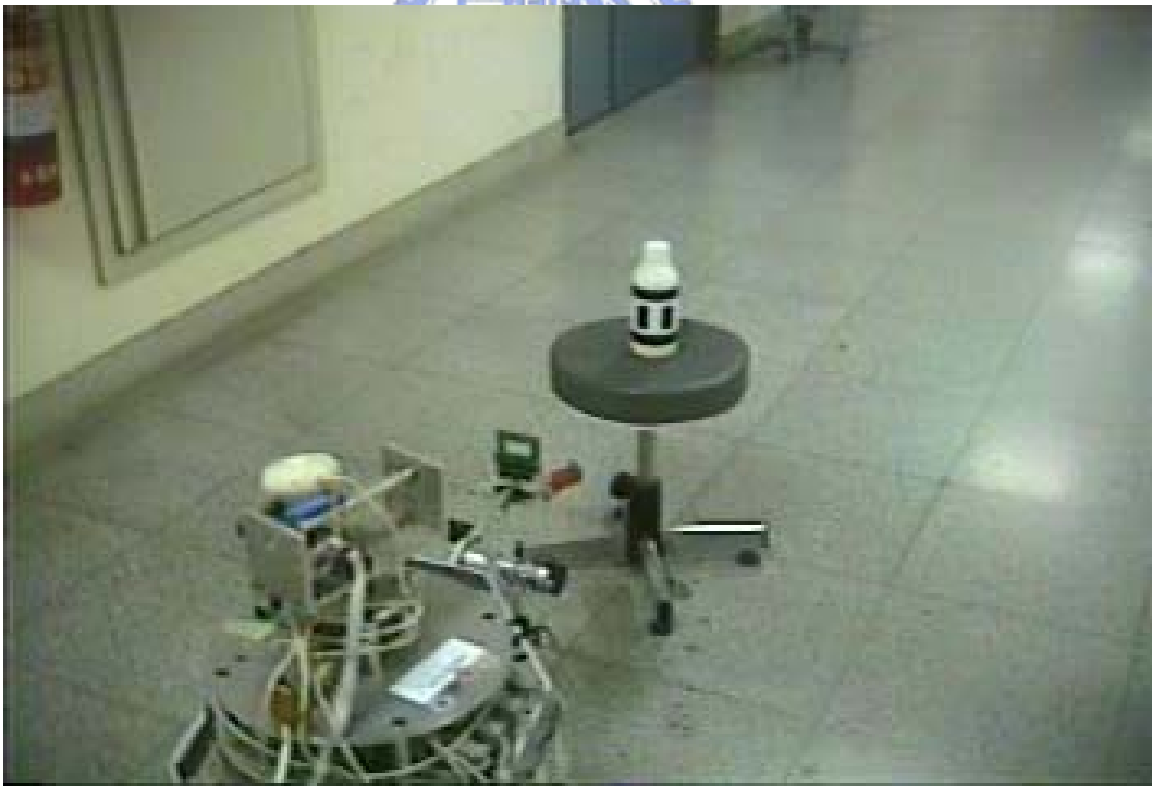
Figure 5.5 (a) the mobile manipulator is approaching the object
