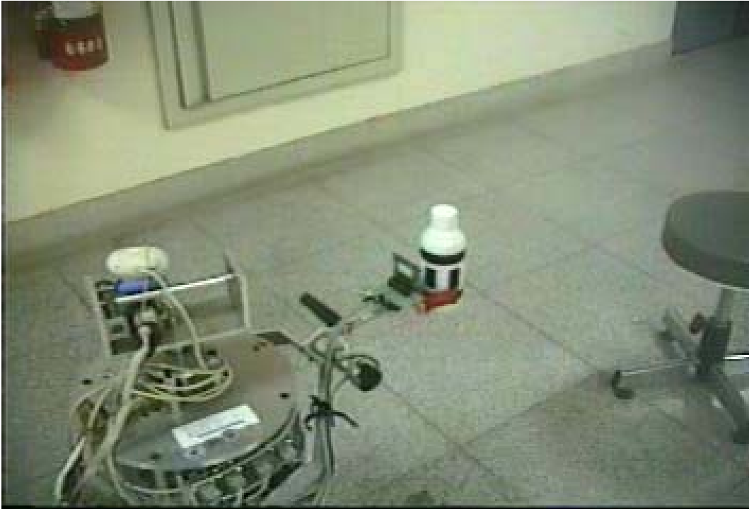
Figure 5.6 (b) the mobile manipulator grasp the object
