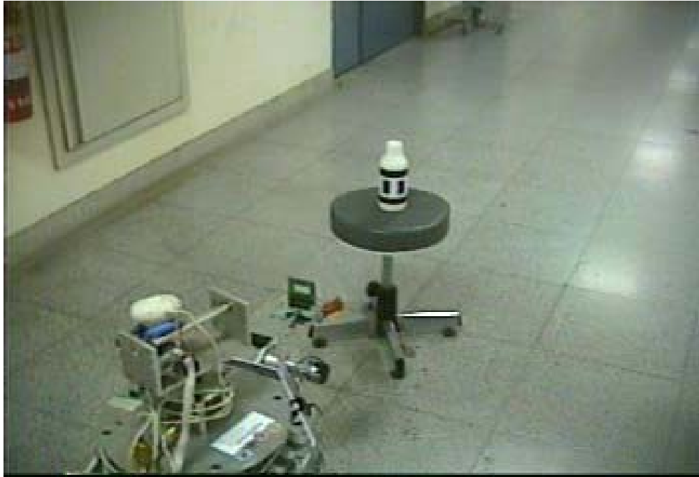
Figure 5.4 the robot change its orientation and speed after it locates the object in front of it
