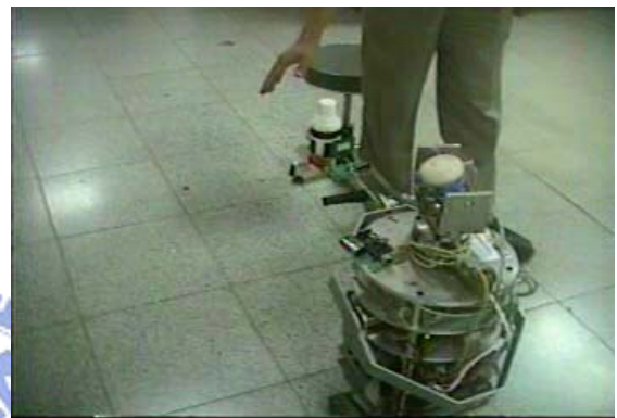
Figure 5.10 (a) the object is in the gripper area Figure 5.10 (b) the gripper grasped the object
