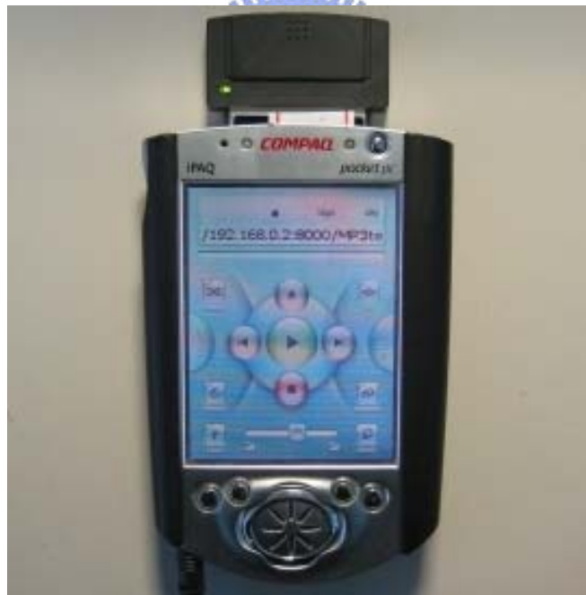
Figure 56. Connects to MP3 Broadcaster Server via PDA
