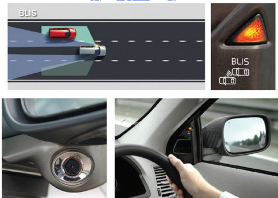
Fig. 2: Volvo Blind Spot Information System
