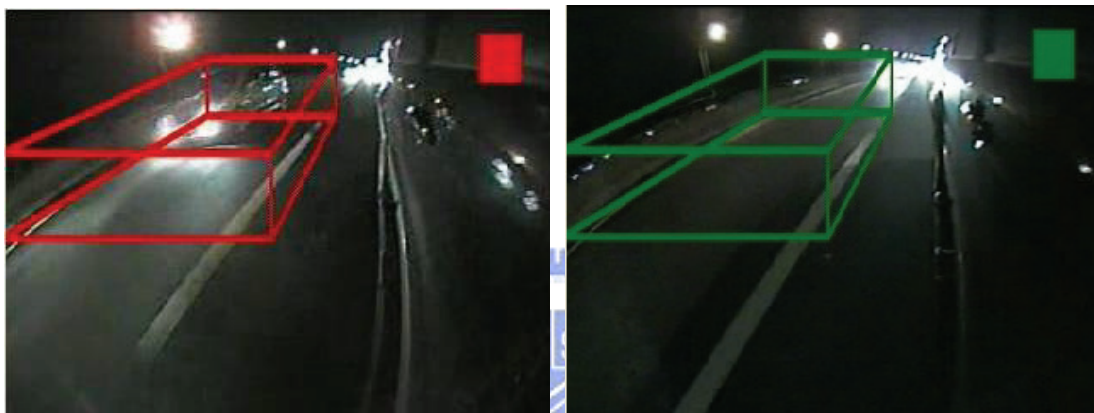
Fig. 39: System won't be affected by the street lamp in the nighttime.
