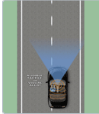
Fig. 1: Delphi Lane Departure Warning System
