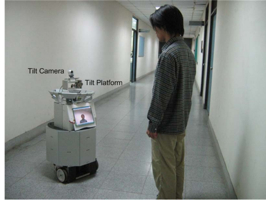
Fig. 5-16: Experimental mobile robot used to test the tracking performance of the proposed VTC combined with the VSE-WoTV presented in Section 4.3.
