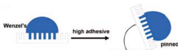
Figure 2.9 The water could permeate into the grooves of the surface. A droplet of water could pin on the replicated surface because of strong capillary forces.
