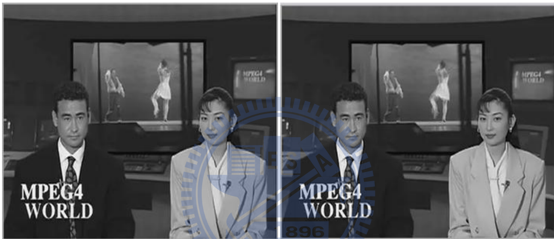
(a) Subjective quality of the 2 nd frame at level 3: WDTM_EC (left): 34.09dB, Proposed (right): 34.29dB, Correct: 36.68dB.
