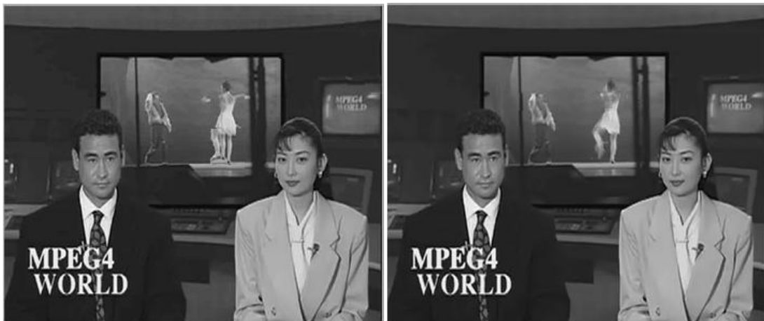
(b) Subjective quality of the 4 th frame at level 2: WDTM_EC (left): 33.88dB, Proposed (right): 35.51dB, Correct: 37.53dB.
