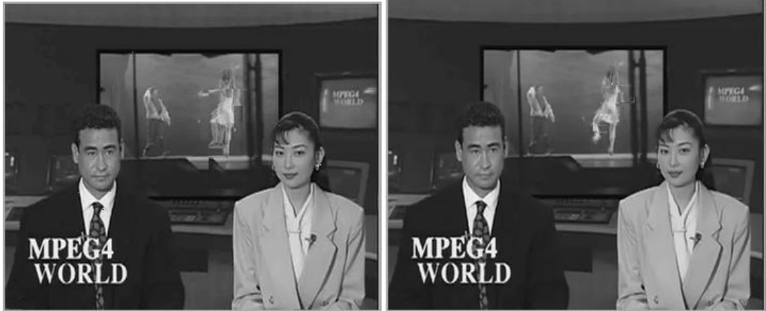
(c) Subjective quality of the 7 th frame at level 1: WDTM_EC (left): 31.33dB, Proposed (right): 34.27dB, Correct: 37.42dB.
