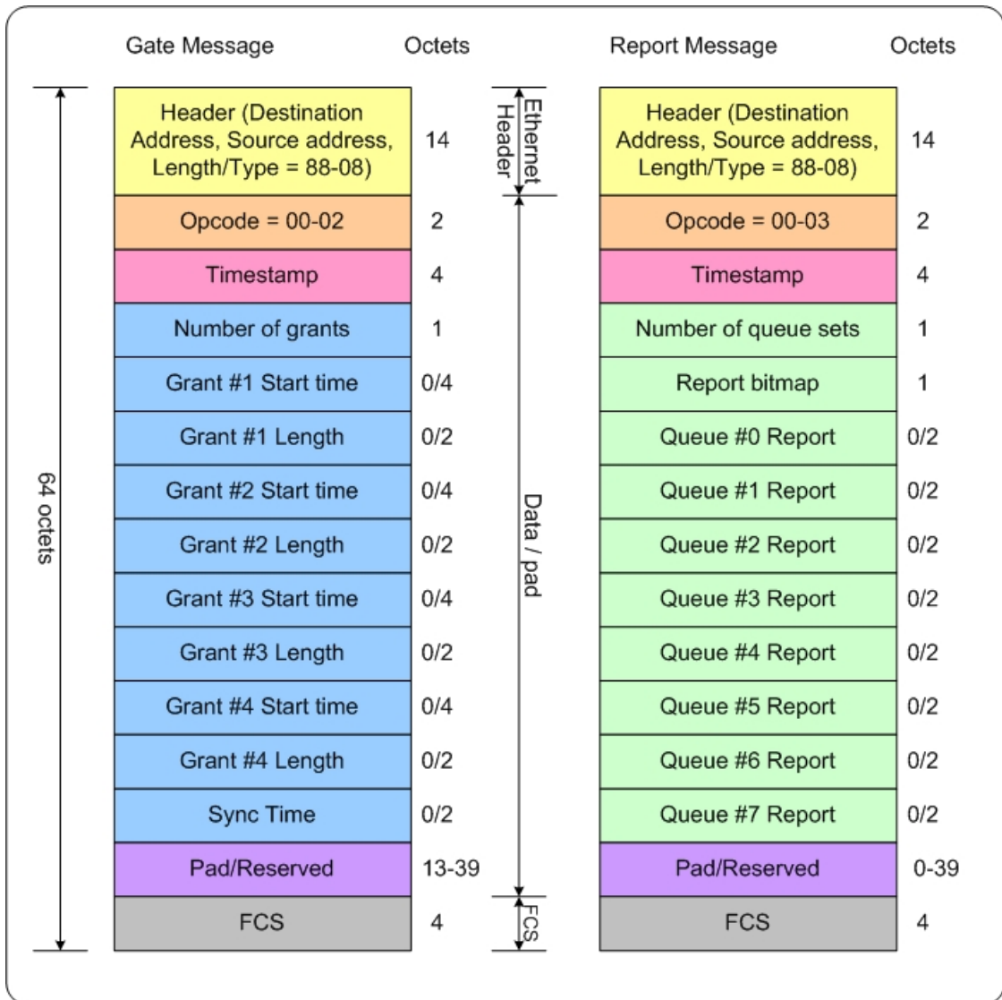
Figure 2.1: GATE message and REPORT message frame format
