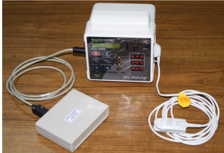
Figure 3-4 Connection of vital sign monitor with WSN end point
