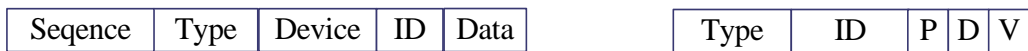
(a) The message sent from WSN end point (b) The message sent from WSN Coordinator
