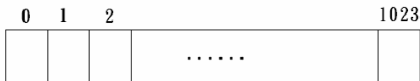
Figure 4-3 fd_set array with fixed size 1024
