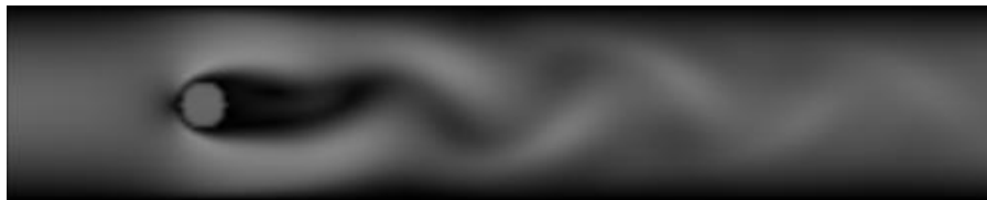
Figure 5.7 The velocity of cross-flow in circular cylinder shows turbulent flow. The dark color represents low velocity, and bright color represents high velocity in flow.
