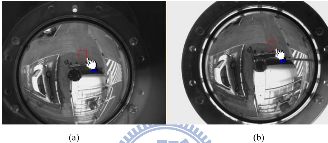
Figure 6.3 The interface for ground learning. (a) The omni-image taken by the upper omni-camera. (b) The omni-image taken by the lower one.
