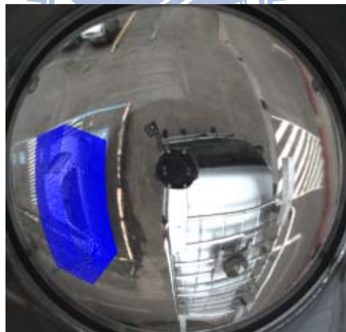
Figure 6.10 An example of cuboid shape placement in an omni-image using forward mapping.
