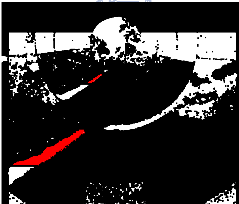
Figure 5.8 The result of detecting the curbstone features in the experimental environment.
