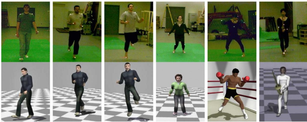
Figure 2.4: The above pictures are that user wearing markers to control the full-body motion of avatar in from of two synchronized cameras. [CH05]
