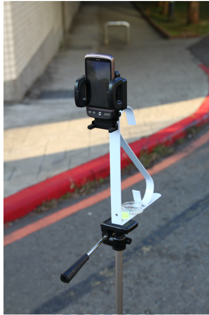
Figure 3.3: The equipment for taking pictures to generate panoramic images
