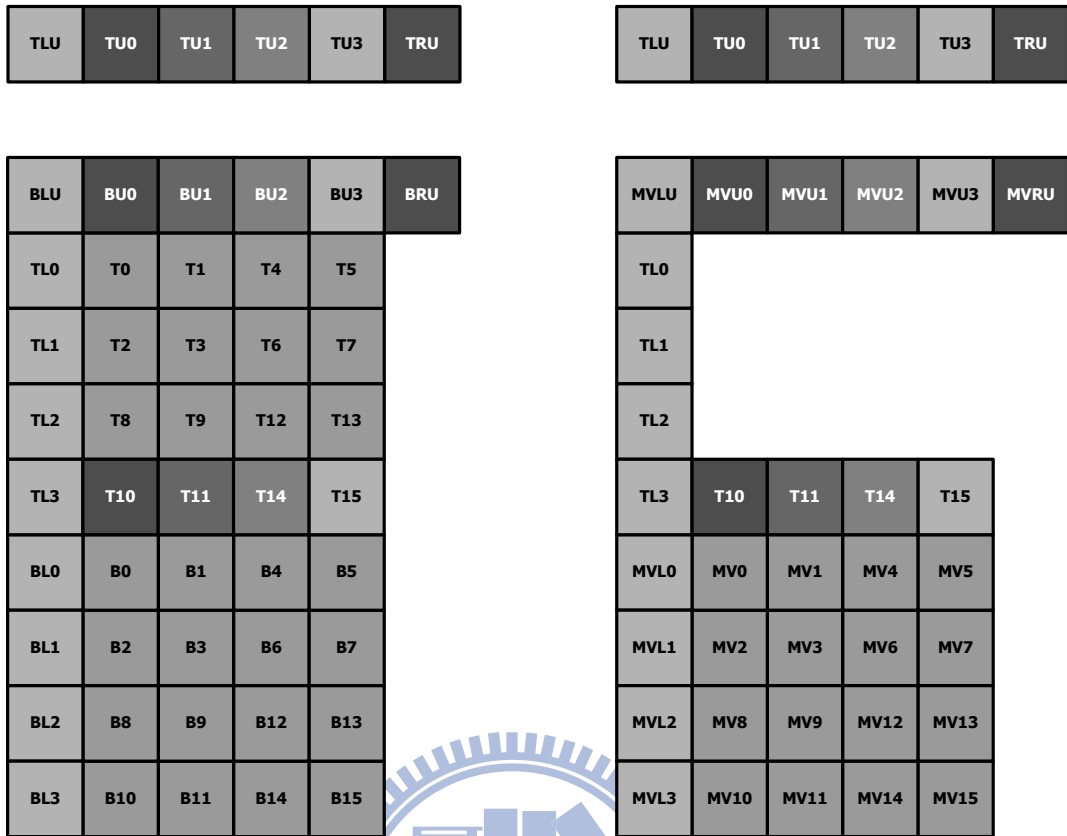
Fig 3.3 (a) Neighboring motion vectors needed when decoding all motion vectors in current MBAFF macroblock, (b) reduced and combined with non-MBAFF version
