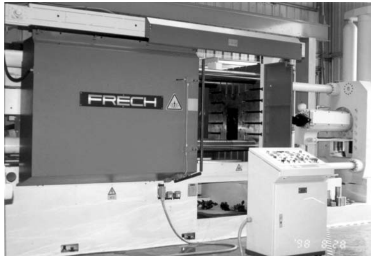
Figure 4.9 Thixocasting machine with clamping force of 5,000 kN
