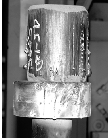
Figure 4.8 Melt beads formed on a semi-solid powder preform
