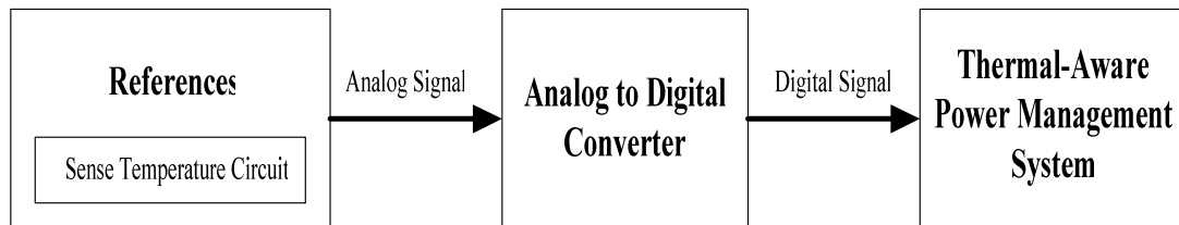
Figure 5.1.1 Building Blocks of Temperature Sensor with TAPM
