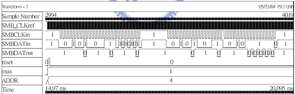
Figure 4.4.5 Testing Controller Register 3 by SMBus (Test Pattern AAh)
