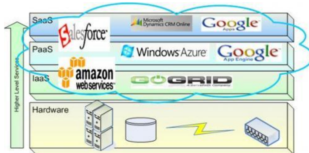
Figure 25: Cloud Computing Architecture. Source from Edgewater Technology
