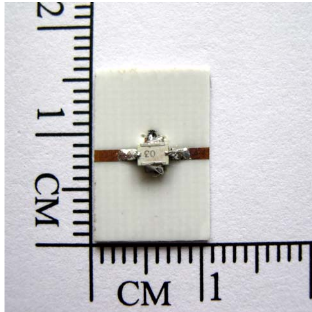
Figure 5.1-7 Photograph of the LTCC combline filter mounted on the substrate
