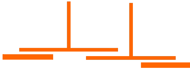
Fig. 3.1-1 (a) Circuit layout of filter of two \lambda/4 UIRs with a tapped stub cascaded by direct coupling structure
