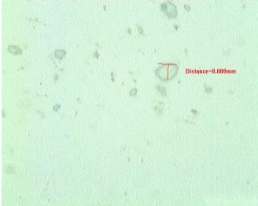
Fig. 4-3 OM image of BCB polymer surface after BCB to thermal oxide bonding at 200 °C/ 30 min
