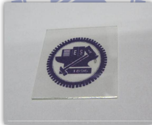
Figure 4-14 Photograph image of a 500°C annealed IGZO thin film on glass substrate placed on a logo.
