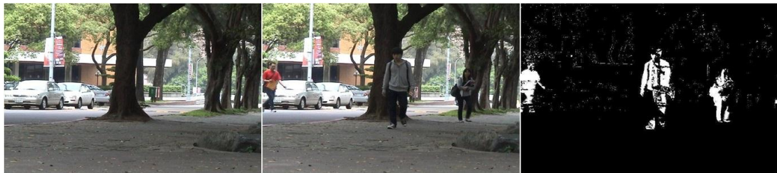
Figure 3-4 The man in the middle of the image walks in front of the tree, but we see the false boundary in the background subtraction result due to the similarity of color.
