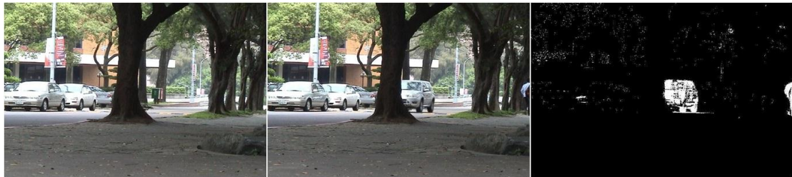
Figure 3-3 When a car passes through the back of the tree, we can see the boundary in the background subtraction result last for a short time.
