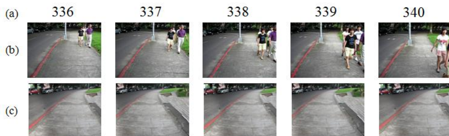
Figure 4-5 Results of database retrieval for walking forward with some pedestrians passing by. (a) Frame index, (b) input frames, and (c) the best match from the panoramic sub-database.
