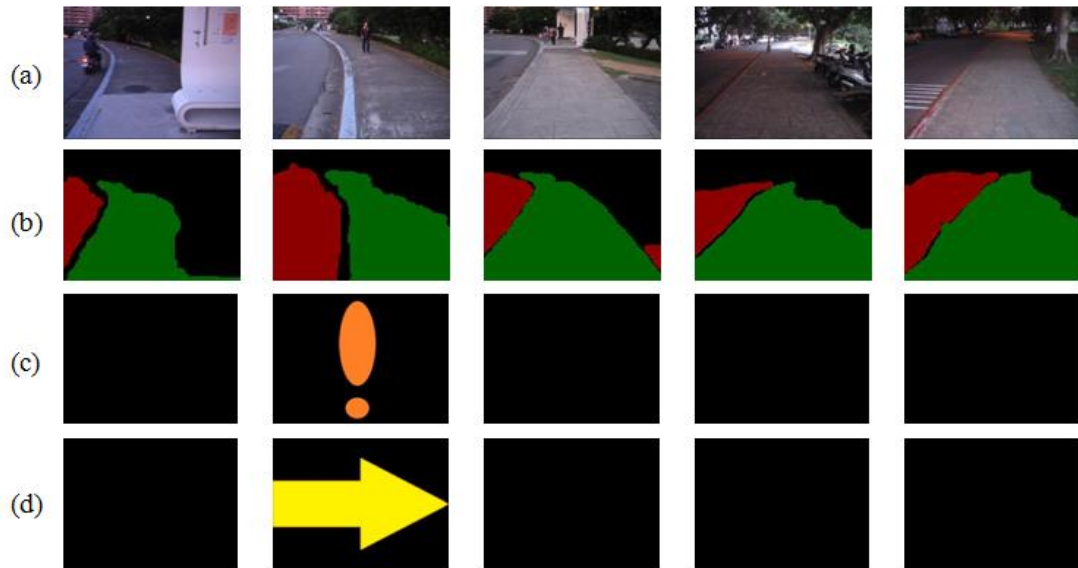
Figure 4-12 Some examples at evening time. (a) Input frame. (b) Inferred labels. (c) Outcome of dangerous situation detection. (d) Suggested turning direction.
