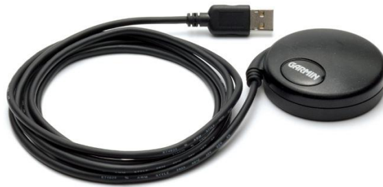
Figure 3-6 Garmin's USB-version GPS 18
