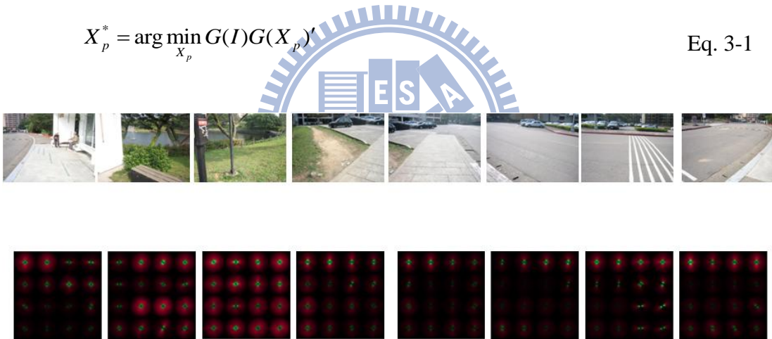
Figure 3-11 Visualization of Gist feature for different image views
