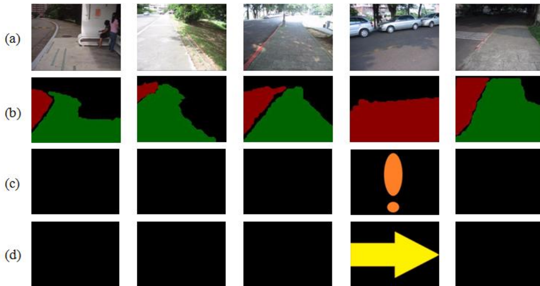
Figure 4-11 Test results in sunny day. (a) Input frames. (b) Inferred label. (c) Outcome of dangerous situation detection. (d) Suggested turning direction.
