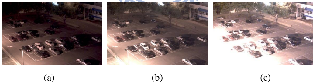
Figure 3-12 (a) The captured image with EV=10 (b) The captured image with EV=50 (c) The captured image with EV=90
