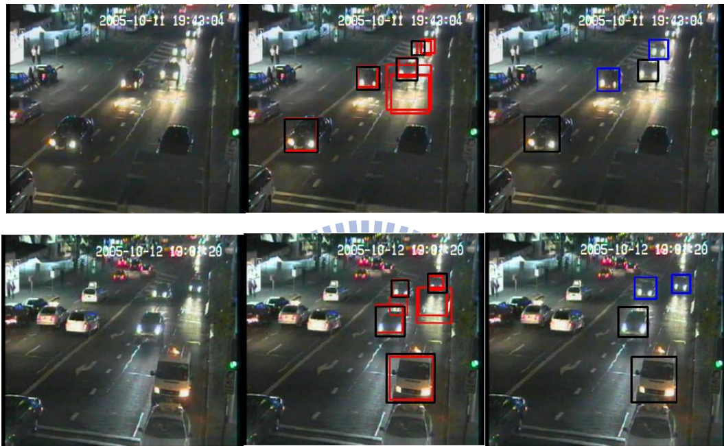
Figure 2-21 (a)(b) Images at night (b)(e) Results from the two-layer detector (red: candidate position, black: detected cars) (c)(f) Results from the AdaBoost cascade detector (blue: missing cars, black: detected cars)
