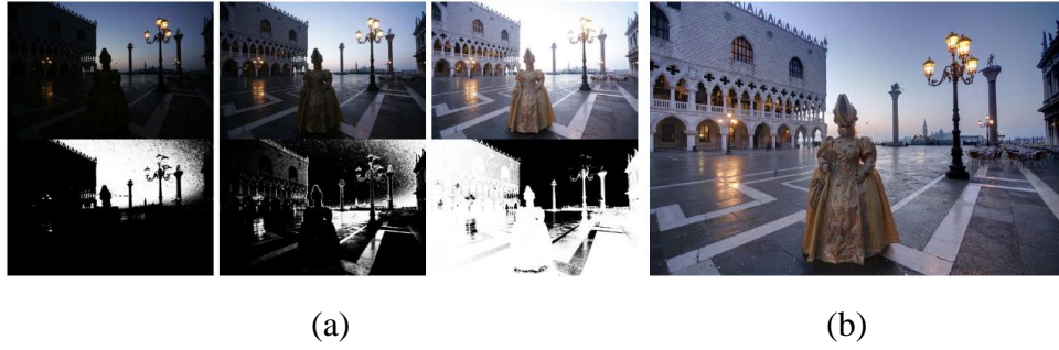
Figure 3-14 (a) An Image sequence and its weighting maps (b) The fusion result
