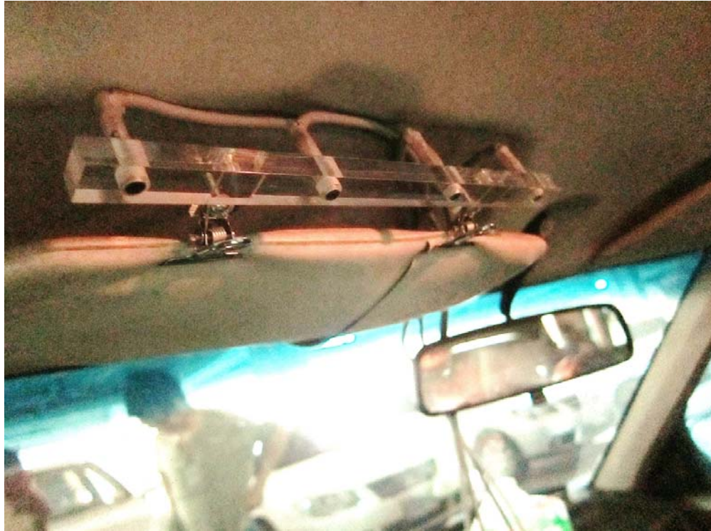
Fig. 10 The photo for the microphone array at the sun shield of the driver's seat.
