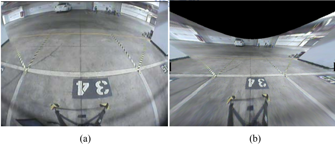
Fig. 3- 6: (a) Original fisheye image and (b) Rectified result.
