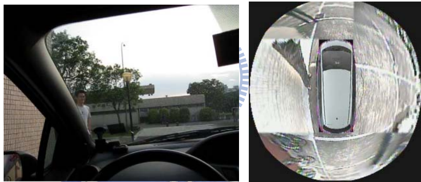
Fig. 2- 4: The bird-eye image of intersection in alley
