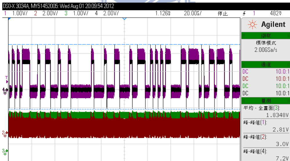
Figure 59. Waveform of coil receive input, demodulated data and baseband data (from signal generator) at 678 kbps with PRBS9 pattern
