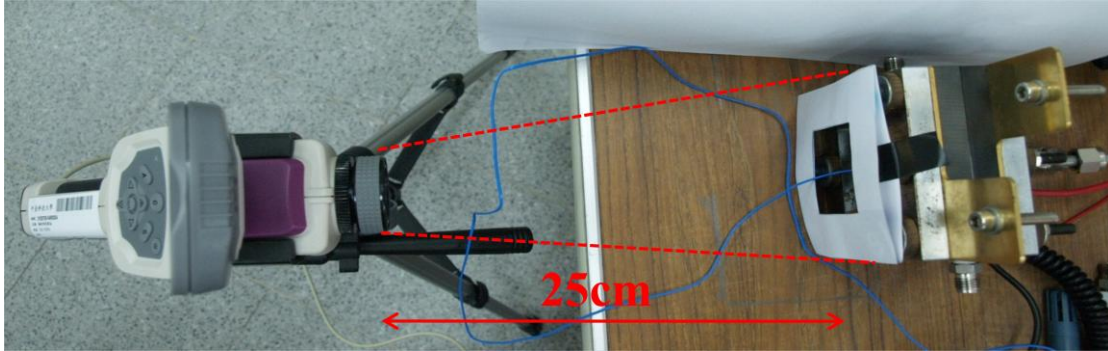
Fig. 3.15 Top View of Thermal Infrared Imaging Camera and Air-breathing Fuel Cell
