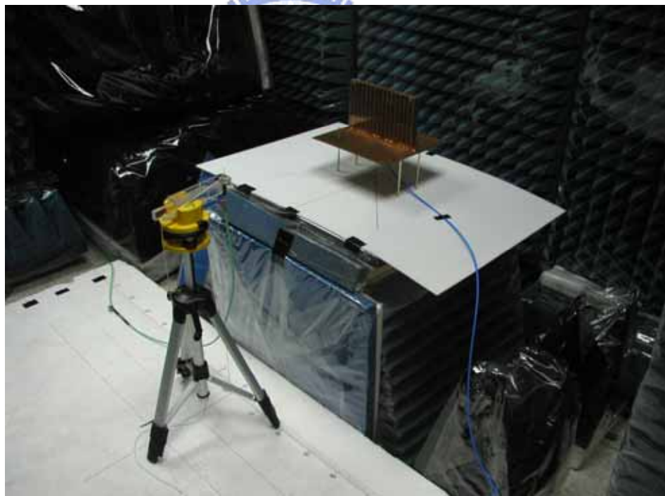
Figure 3: (a) Measurement setup in chamber (b) The probe is at the position (x, y, z) = (0, 0, 52)
