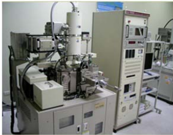
Fig. 2-5: EBL system (ELS - 7500EX), facilities of CNST , NCTU .
