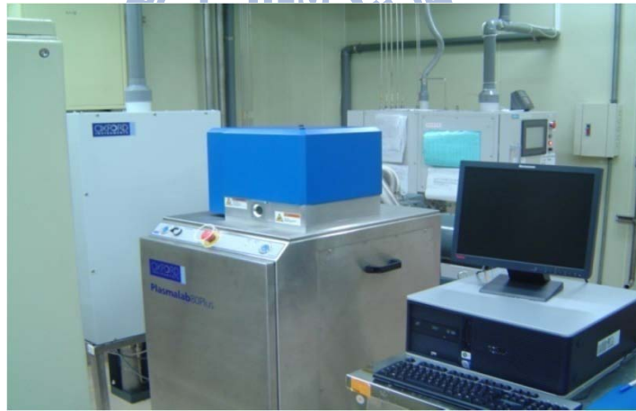
Fig. 2-4: Picture of PECVD system (Oxford Instruments Plasma Technology Plasmalab 80 Plus), facilities of Center for Nano-Science and Technology ( CNST ), National Chiao Tung University ( NCTU ).
