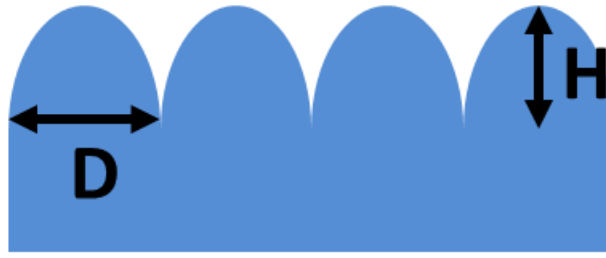
Figure 5-1 Illustrations of the definition of the height and bottom width of nanostructure.
