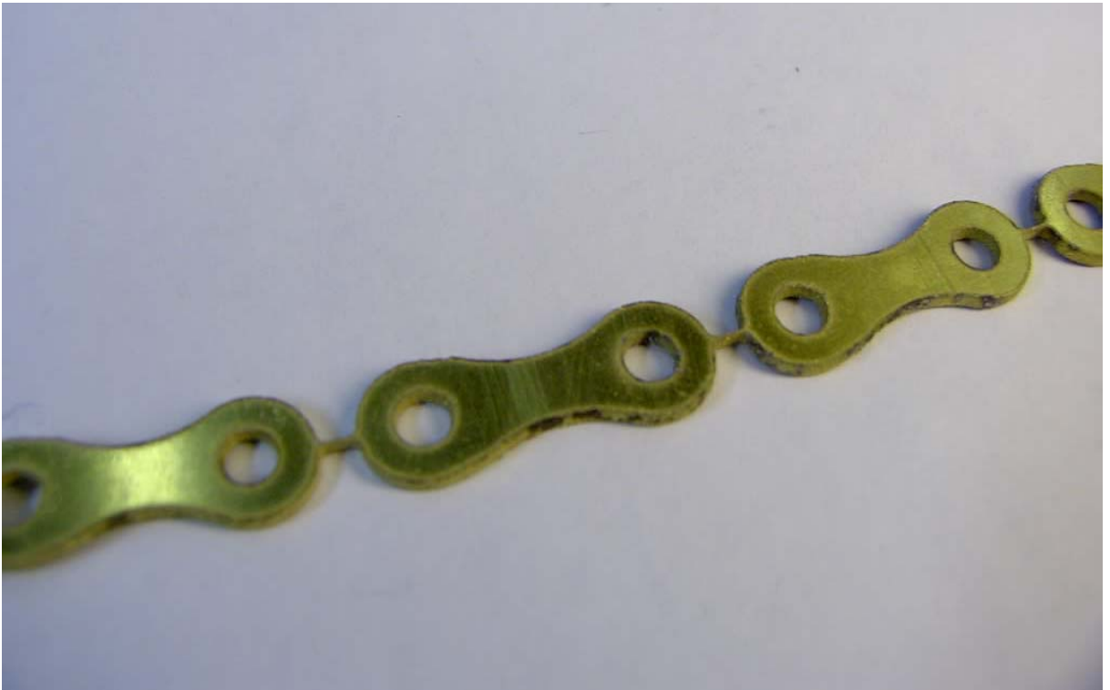
Fig. 5.2 Chain plates manufactured by water jet
