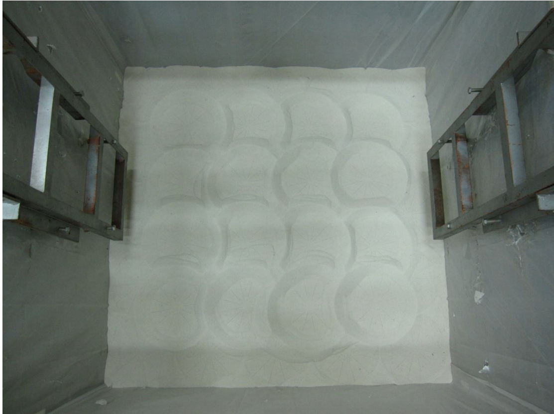
Fig. 6.23. Compacted soil surface after 4×4 formation of cyclic torsional shear at N=5
