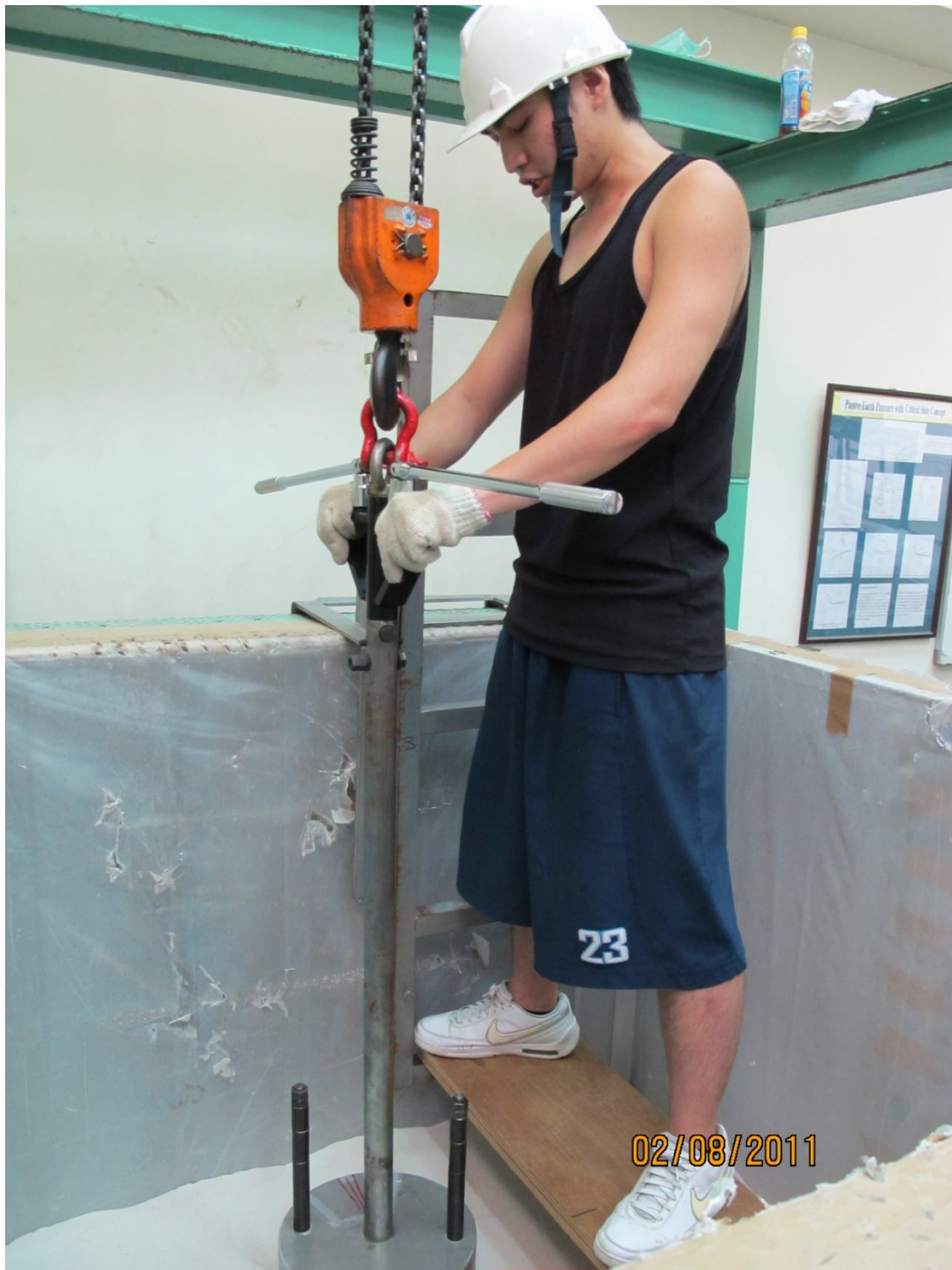
Fig. 6.13. Hoist of CTSC with overhead crank
