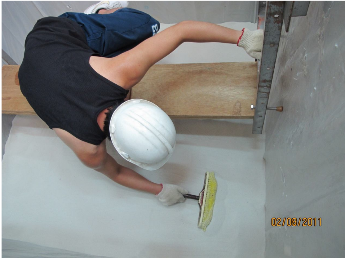
Fig. 6.6. Level soil surface with a brush
