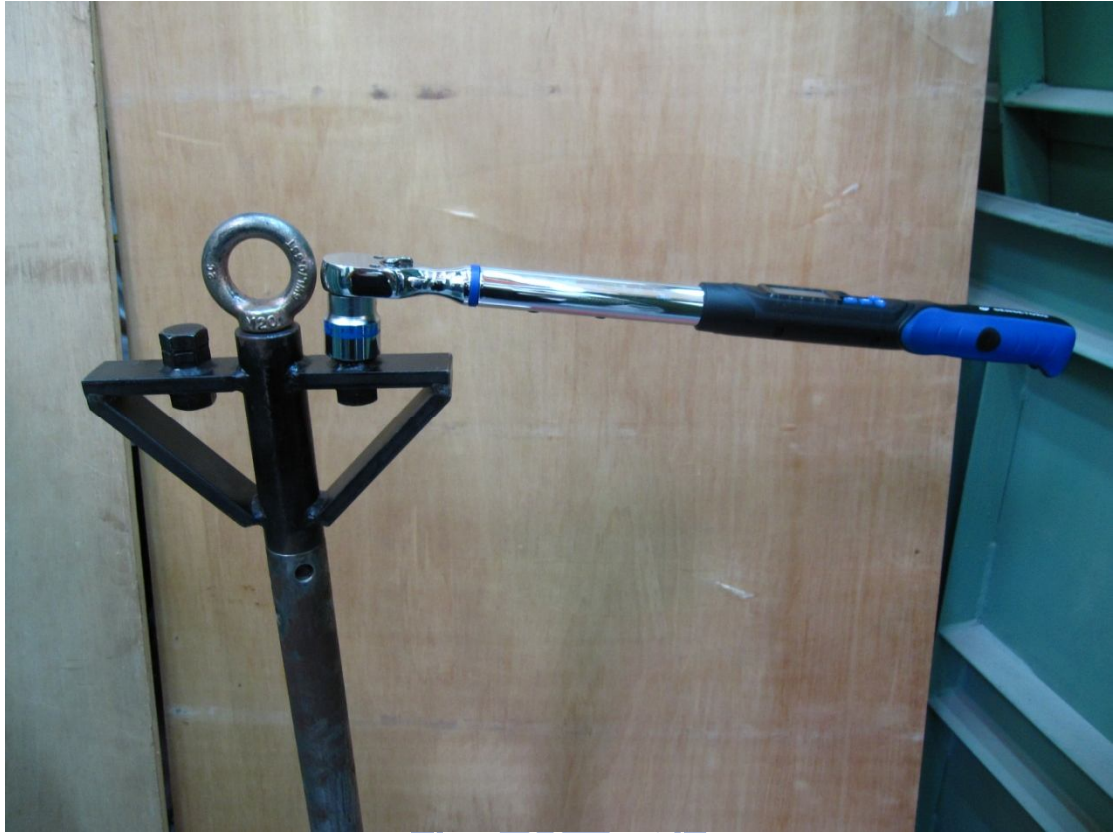
Fig. 4.12. Torque wrench are installed on the cyclic torsional loading frame
