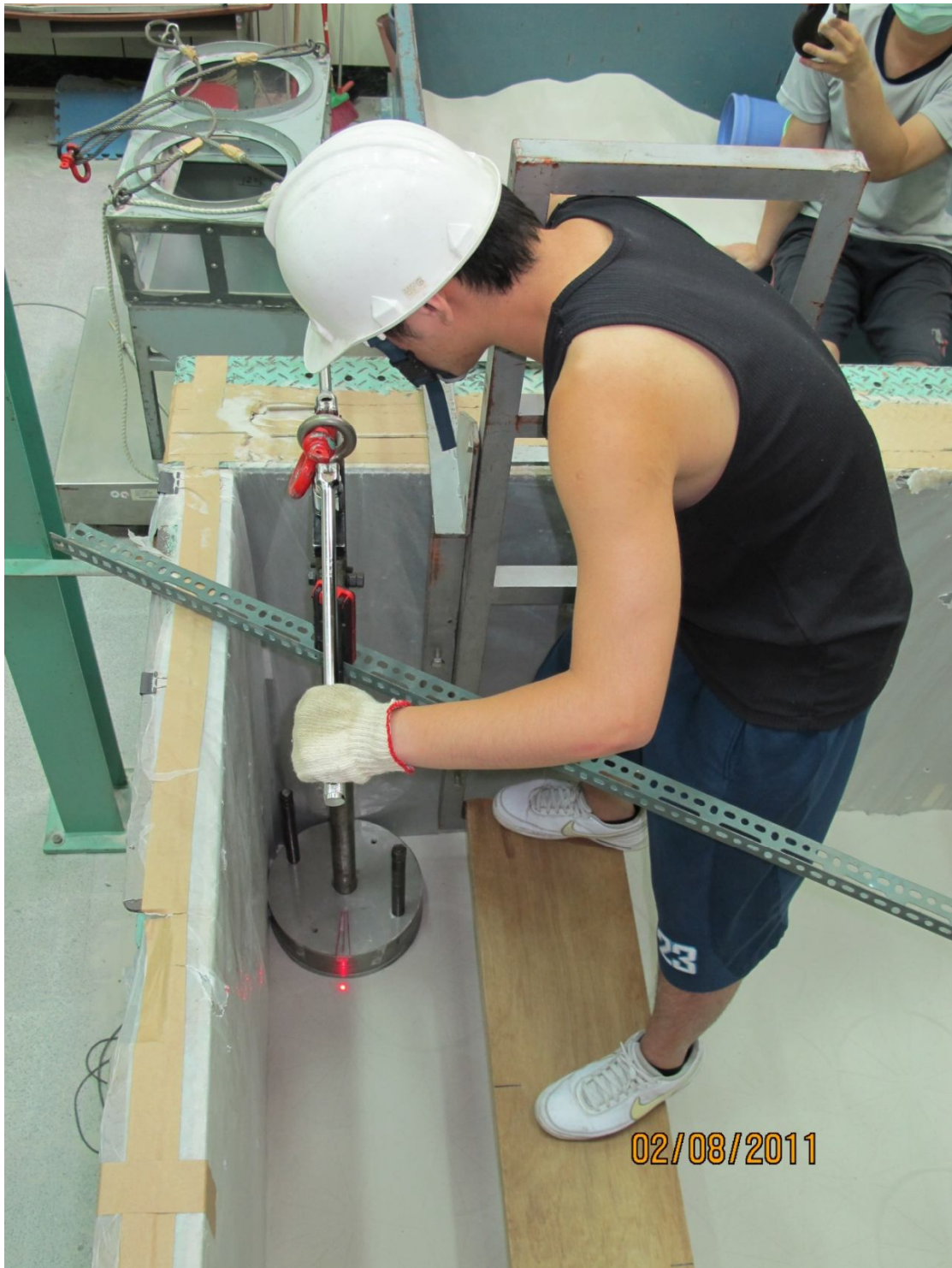
Fig. 6.18. Apply cyclic torsional shear on loose fill
