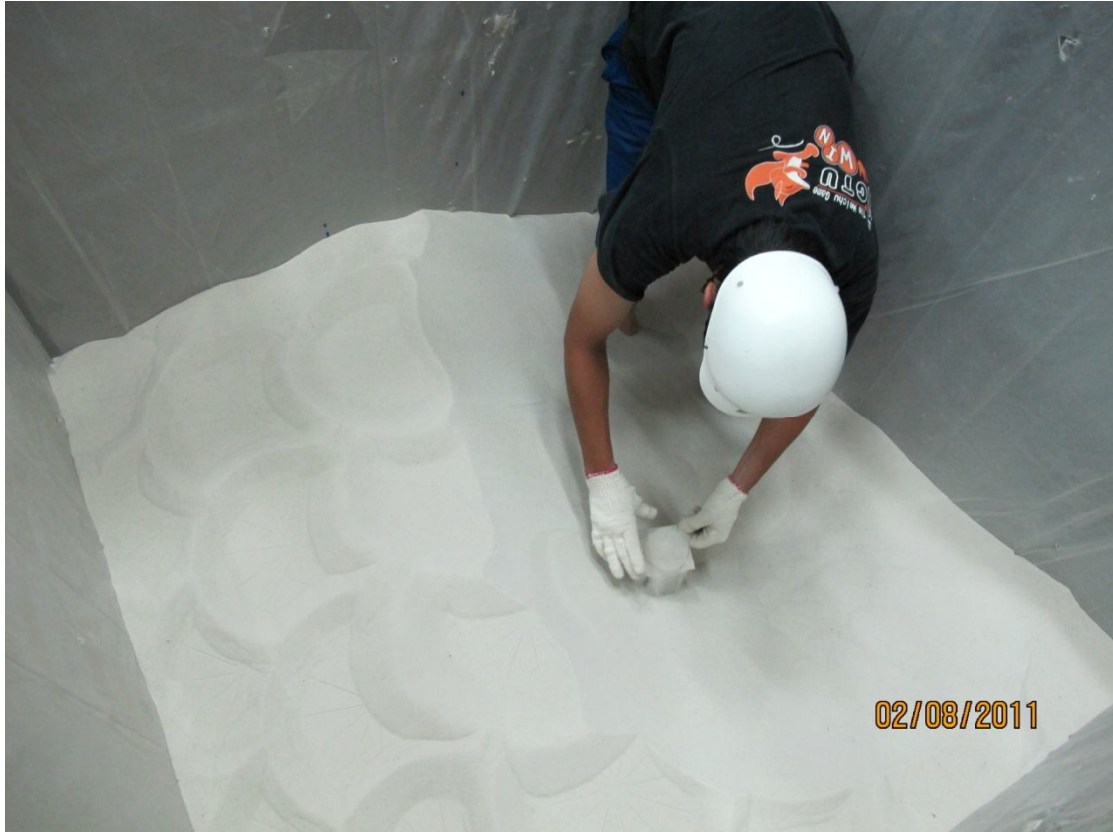
Fig. 6.25. Soil density cup dug out of compacted soil mass
