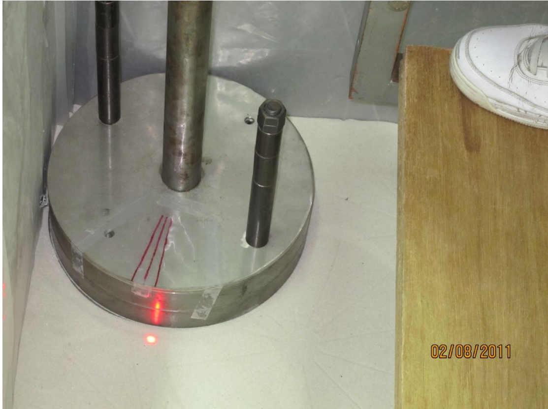
Fig. 6.21. Shear disc rotated to \theta = -5^\circ
