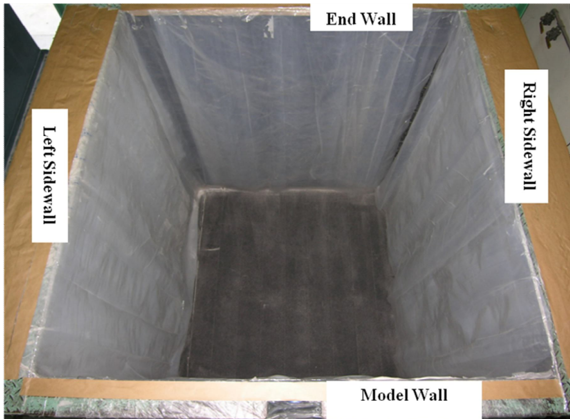
Fig. 5.2. Lubrication layer on the side wall
