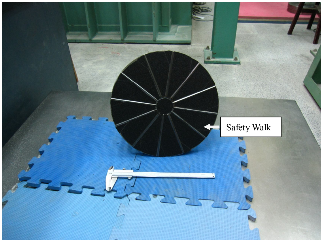
Fig. 4.5. Bottom of shearing disc with SAFETY WALK
