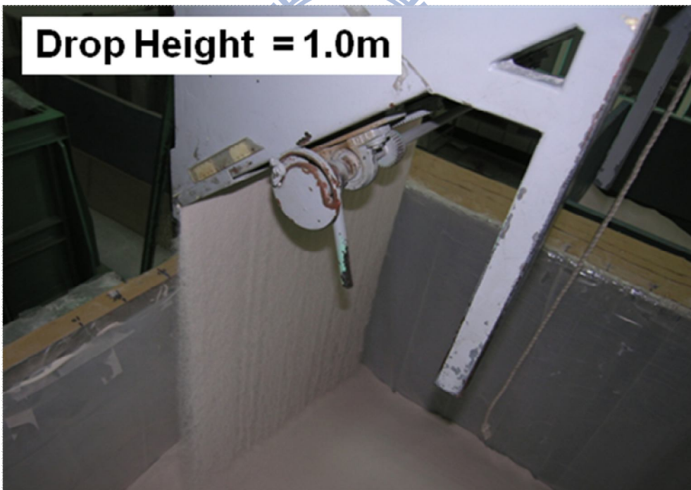
Fig. 5.6 Pluviation of Ottawa sand into soil bin
