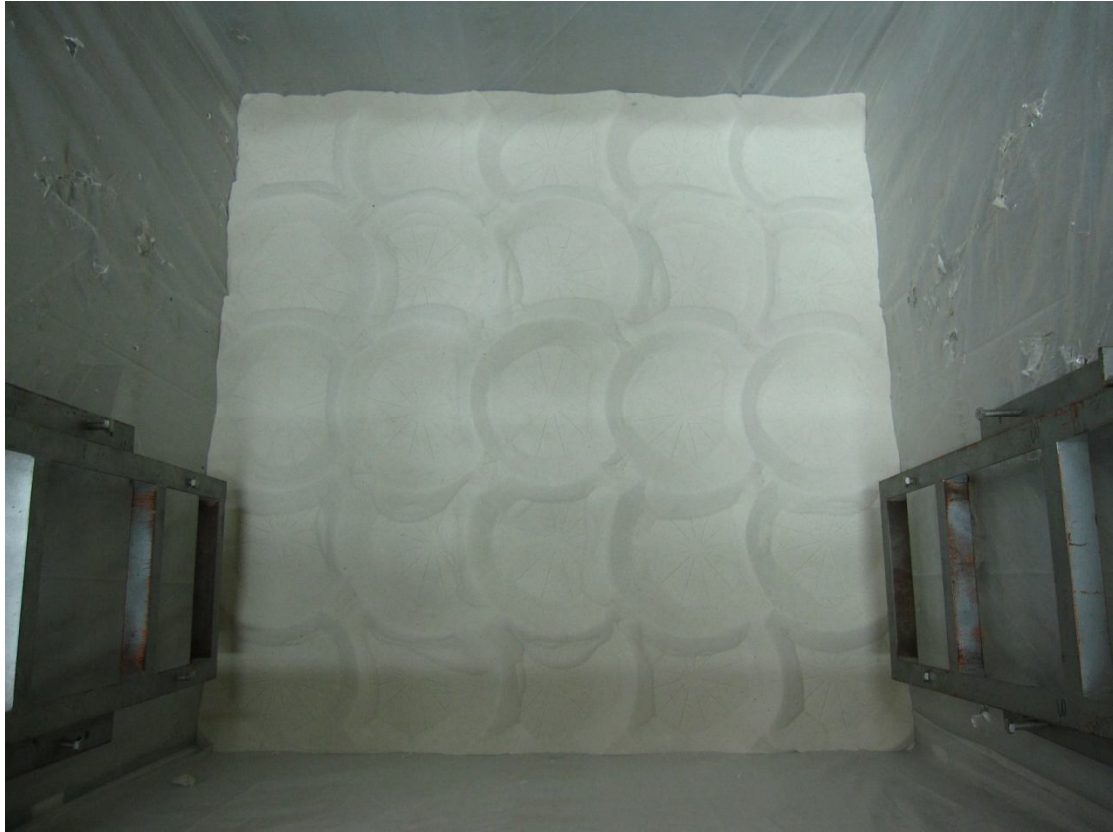
Fig. 6.24. Compacted soil surface after 5×5 formation of cyclic torsional shear at
