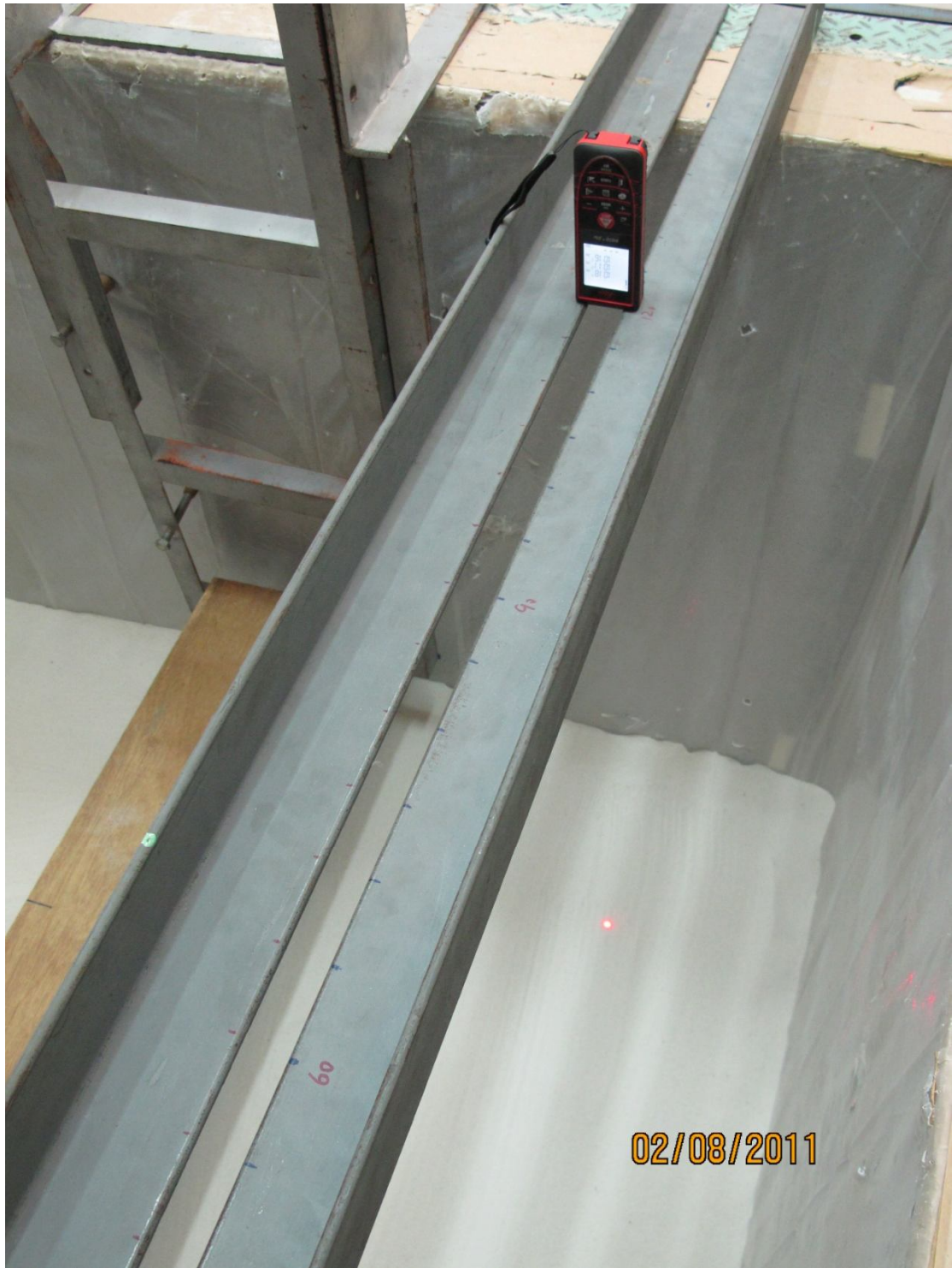
Fig. 7.9. Settlement measurement was carried out with the laser distance meter
