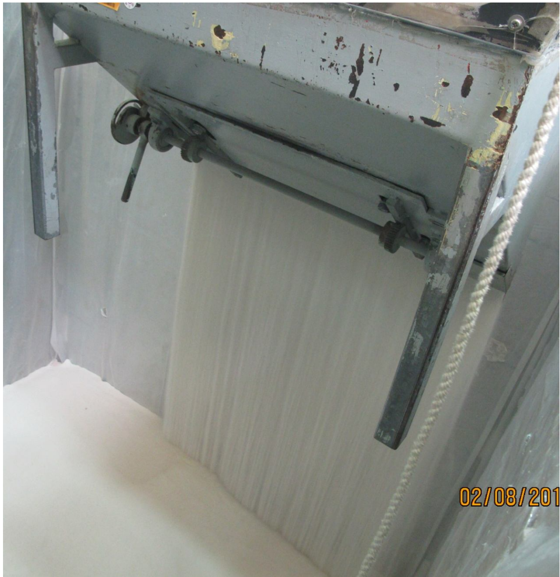
Fig. 6.4. Air-pluviation of Ottawa sand into soil bin
