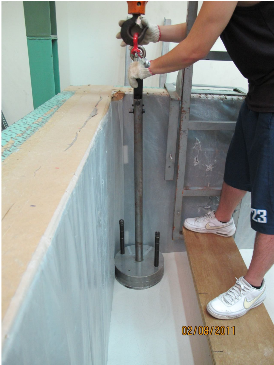
Fig. 6.15. Apply vertical static load on loose sand
