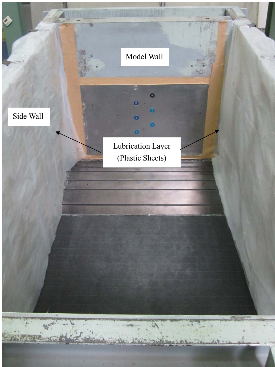
Fig. 5.6. Plastic-sheet lubrication layers on side walls
