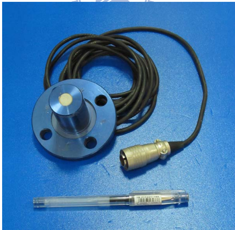
Fig. 3.6. Soil pressure transducer (Kyowa PGM-0.2KG)
