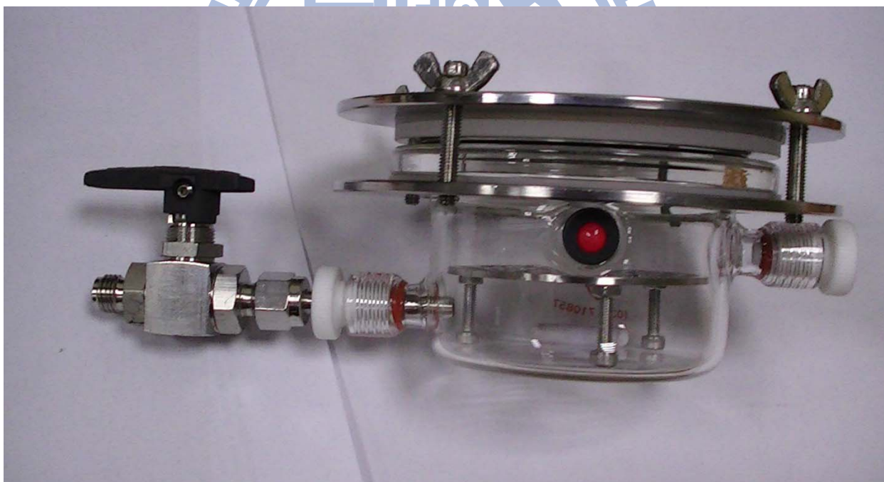
Figure 3-1 A photograph of the reactor for photocatalytic reduction.
