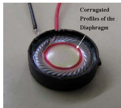
Fig. 2 Corrugated profiles of the diaphragm in the micro-speaker
