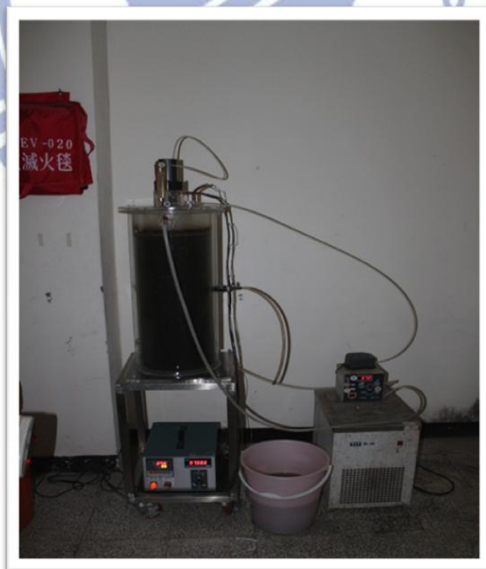
Fig. 5. Photograph of SBR
