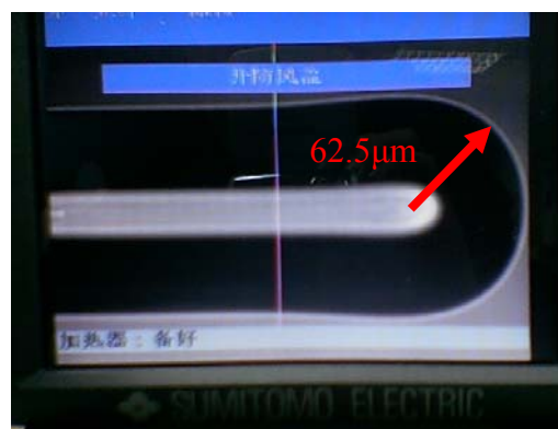
Fig.4-14 Photograph of fiberlens with radius 62.5 \mu\text{m}
