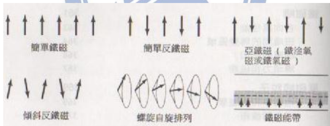
Fig. 2.7 Ordered arrangements in electron spins.
