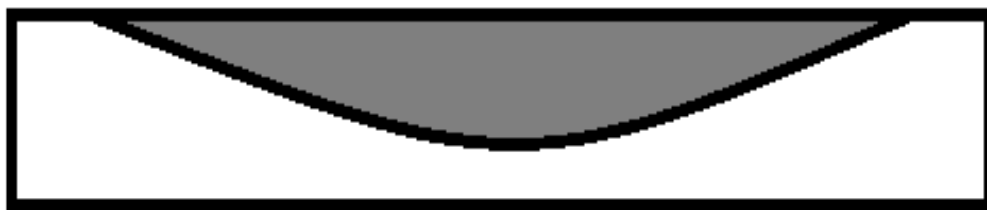
Fig. 5-7 The shadow part is ablation region. It causes spatial dependence of the linear refractive index n_0 . When sample is brought closer to the focus, most part of beam begins to diffract and produce intensity variation in far field.
