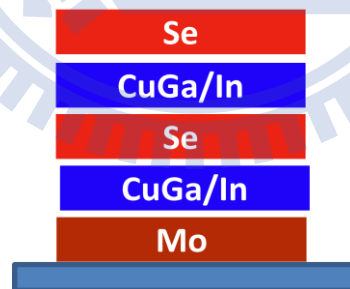
Fig. 4-16 The modified structure.
